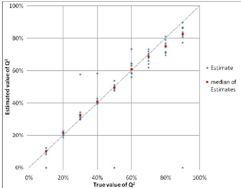
Figure 4: Monte Carlo Simulation results for nine values of  $Q^2$  with ten repetitions each. The EM-MLE estimates are compared to known true values. The circles indicate the median values of the estimates. Estimates lying on the  $45^\circ$  are exactly equal to the true value.
